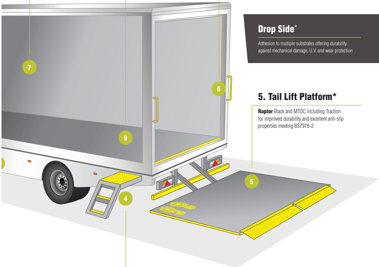
\*To aid adhesion and extend the life of Raptor on bare metal substrates, use Raptor Epoxy Primer to give you optimal anti-corrosive protection and excellent salt spray resistance.
