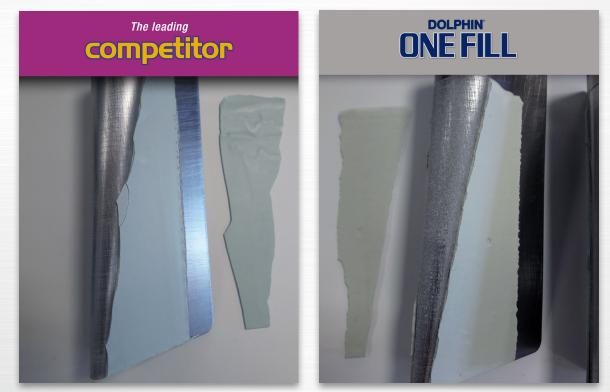
\* Testing conducted in accordance with ASTM D-1002 Lap Shear Adhesion Strength Specifications. When flexed and stressed to failure, Dolphin ONE FILL breaks clean and straight vs. the competitor's uneven break. This test demonstrates that Dolphin ONE FILL adheres stronger than the competitor product.
