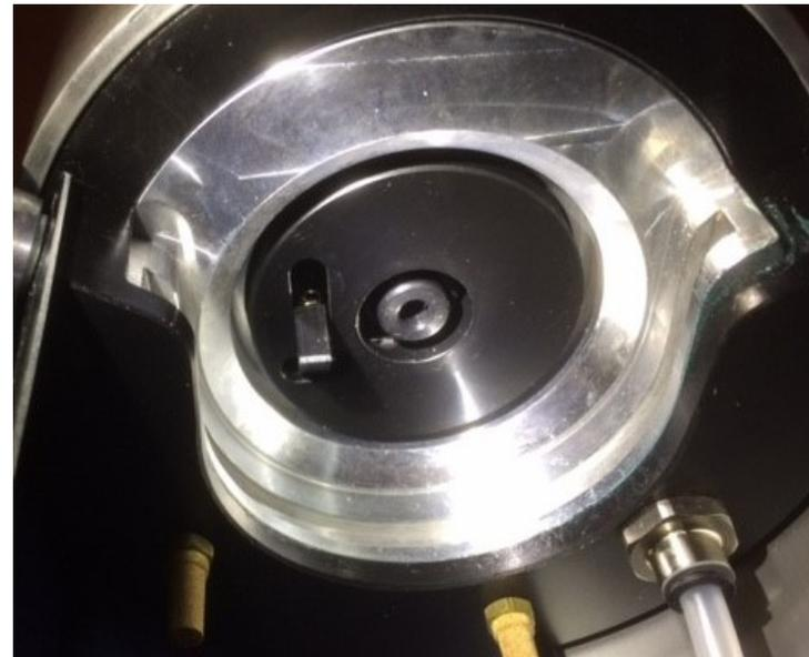
Poorly maintained piston head has paint build up in grooves, preventing proper disc seating
